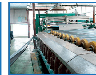
Calender Machine for PVC Sheet Production
