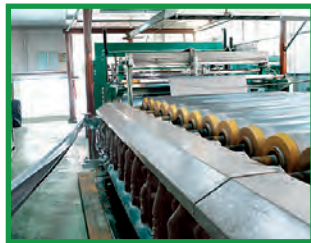
Calender Machine for PVC Sheet Production
