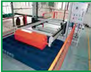
Dynamic durability test for airmattress.
